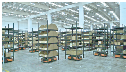
Intelligent robots automatically pick and transport goods in warehouses
